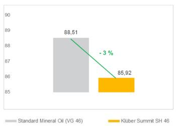
[Test parameters: screw-type compressor; output pressure 7.5 bar; discharge temperature 85 °C; input pressure atmospheric, input temperature 15 °C]
